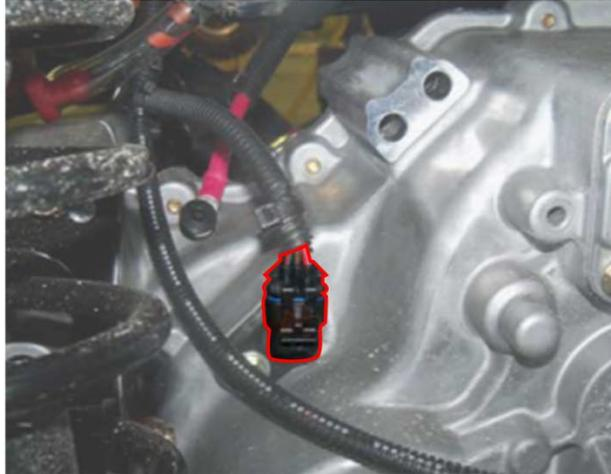
**Step 2:** Connect blue wire from wire harness (3) to red with green stripe wire, then secure the wire harness with electrical tape ensure no interference with other components.
