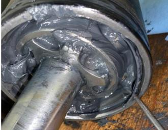
• Pull the full assembly (race, cage, balls) out and locate the snap ring on top of the race
