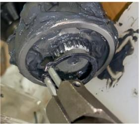
Pull the race assembly out to remove the boot
