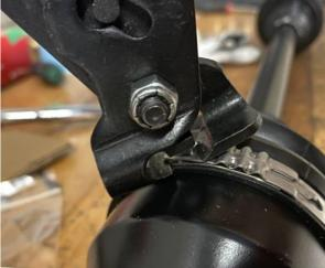
• For reusable clamp, squeeze the tension hook to unsnap the clamp
