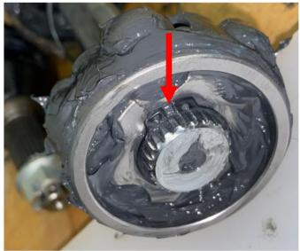
• Expand the snap ring with a snapring plier, then remove the snap ring
