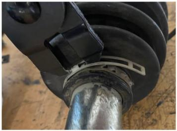
• Pull down the boot and wipe out the crease untill the metal surface is exposed
