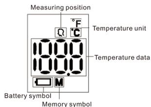
Location indication: The icon flashes to indicate the correct measuring position when measuring.
