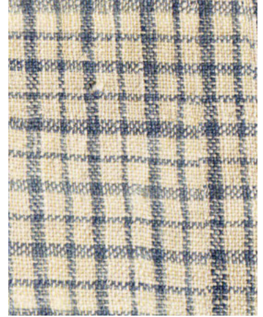
A fragment of an American mid-C19th linen and wool plain weave, indigo dyed.
