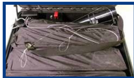
Figure 23B. Launch Tube Lines Before Attachment to Drogue
