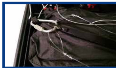
Figure 23C. Launch Tube Attached to Drogue Clip
