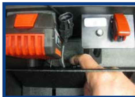
Figure 24. Locate Reset Button Facing the Power Switch
