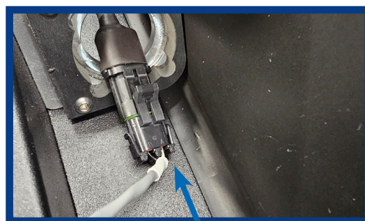
Figure 20. Launch Tube Electrical Connector
