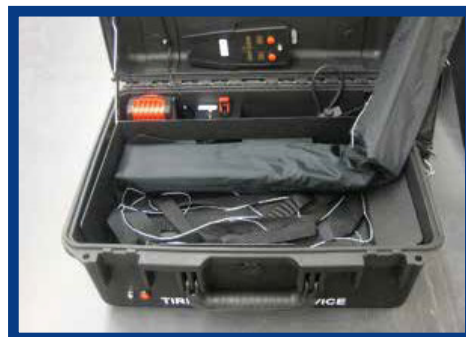
Figure 16. First Spike strip With Tether to the Left Side
