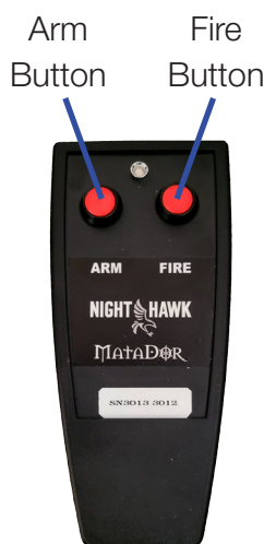
Figure 10. Hand Held Remote Press and hold Arm Button then press and release Fire Button to launch spike strips
