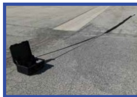
Figure 11. Extended Sleeve and Drogue
