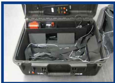
Figure 15. Tether and Retraction String Layered in Tray
