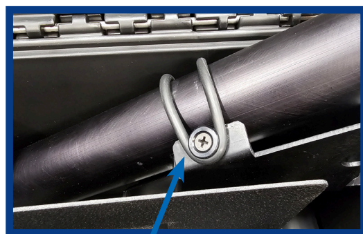
Figure 21A. Launch Tube Anchor Strap
