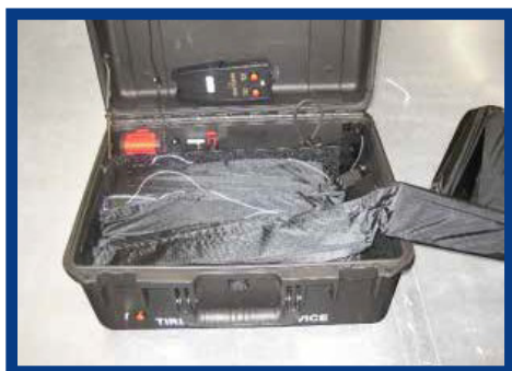
Figure 17. Spike strips Layered in Tray in Alternating Fashion
