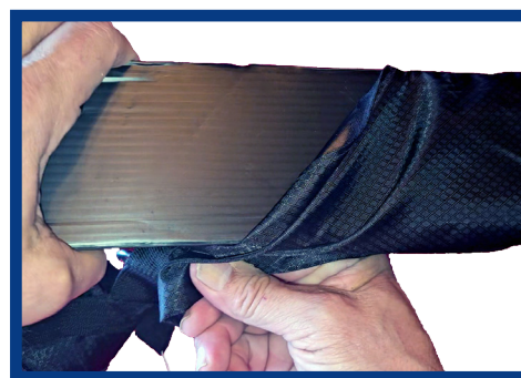
Figure 13B. Replacing Spike Strips
