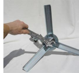
**Aligning the Grip Head with One Leg:**
