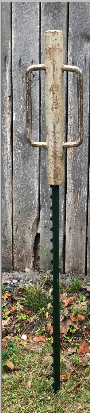
T-Post and Driver – t-post blade has been driven beneath ground surface.
