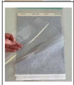
The finished unit of template and Spirit Mater is now placed in the carrier. The white cover sheet is on top!
