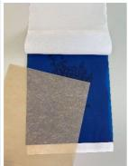
Remove the light brown release paper between the wax layer and the white cover sheet. This cover sheet bears a colored copy of the template on the inside after the successful copying process.
