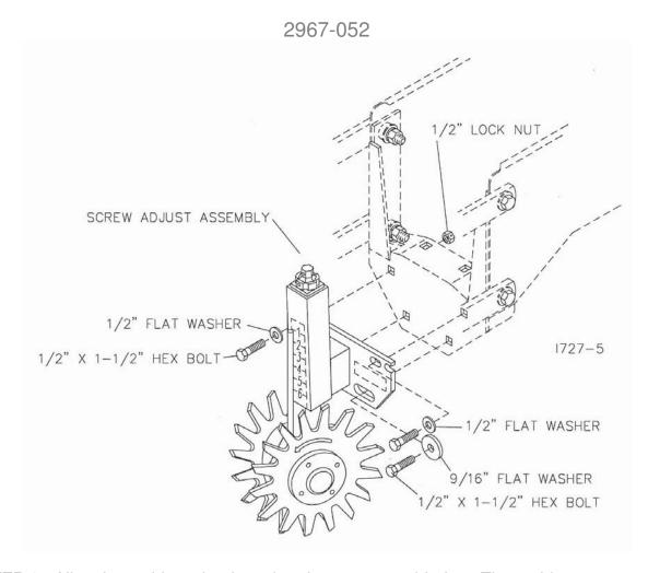
**STEP 3.** Align the residue wheels to the planter opener blades. The residue manager mount bracket has slotted holes in the faceplate to move the residue manager wheels side to side; to be able to center the wheels on the furrow. Fully tighten mounting bolts. Torque to 85 ft. lbs.
