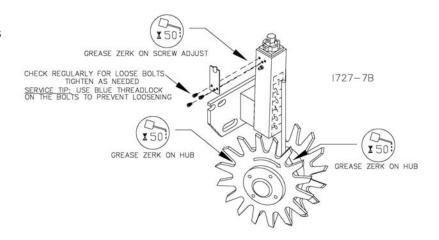
IMPORTANT: The recommended service intervals are based on normal conditions; severe or unusual conditions may require more frequent lubrication.
