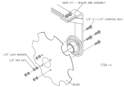
**STEP 4.** "Barn Yard Setting" – set the sealer blade to 2" closer to the bottom of the knife than the depth that the knife will be used at. Example: knife at 6" depth, set the blades to 4" above the bottom of the knife. Adjust the blade pitch as needed to cover the knife track with soil. Tighten all hardware to the recommended amount of torque unless otherwise stated.
