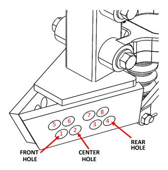
As shown in the picture, Each Stem's side plate has two rows of holes (8 holes total). One of the holes on each side must be selected based on your soil condition and your planter manufacturer to attach the wheel assembly to the stem.
