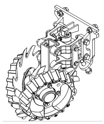
SHOWN WITH OPTIONAL SmartClean CYLINDER (SC-CYL-2X2) and RTW14125-L/R4 Razor Wheels
