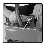
2) Hook the spring onto the hole in the mounting plate and connect it to the bolt on the control arm.
