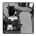
2) Fill the engine with 10W - 30 engine oil.
