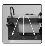
**2)** Install 2 d-ring tiedowns on each side of the frame using the supplied nuts and holts.
