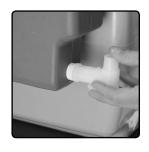
**4)** Before starting your engine, make sure the pressure regulator is fully open (counter clockwise) to avoid premature wear or damage to the pump.
