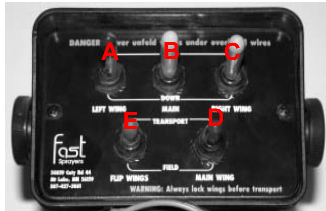
Fig. 1 WING CONTROLS (5 FUNCTION BOX)
