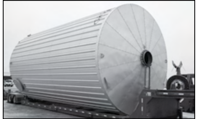
Fig 17 - Insulation and Galvalume Cladding:
