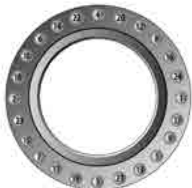
Fig 29 - 24 Bolt sequence
