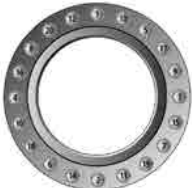
Fig 28 - 20 Bolt sequence
