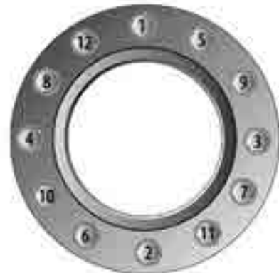
Fig 26 - 12 Bolt sequence
