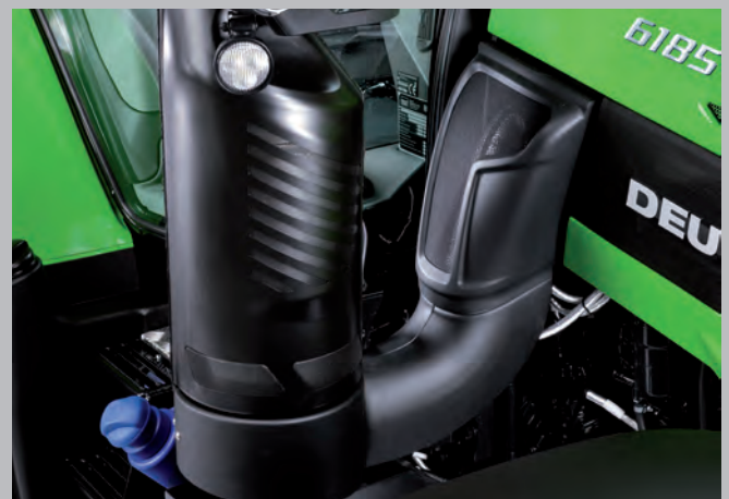
SCR after treatment system and passive DPF (diesel particulate filter) save fuel and costs.
