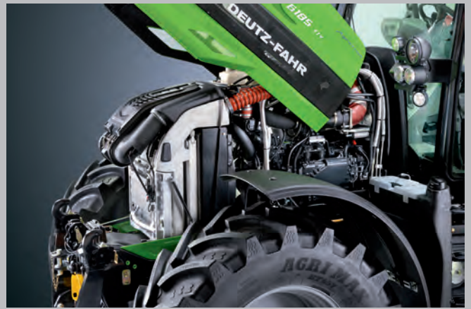
Efficient and compact cooling system for inter cooler, engine, transmission and fuel cooler, and air conditioning condenser.
