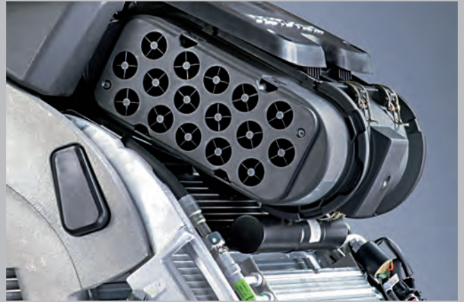
Precleaning system of the air intake filter: spiral tubes and an aspirator hose removes 95% of the dust before entering the primary filter.
