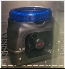
Comments: Device passed test with no negative reaction. The unit worked both at beginning of test cycle and after testing was complete. A periodic function test was run during the testing procedure.
