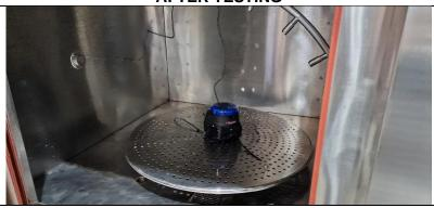
Comments: Device passed test with no negative reaction. Lamp worked both at beginning of test cycle, during and after test cycle complete.
