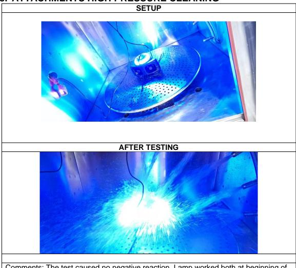
Comments: The test caused no negative reaction. Lamp worked both at beginning of test cycle, during and after test cycle complete.
