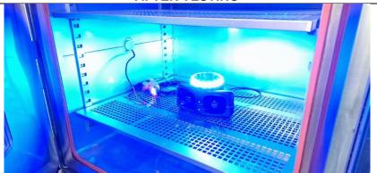
Comments: Device passed test with no negative reaction. The unit worked both at beginning of test cycle and after testing was complete. A periodic function test was run during the testing procedure.
