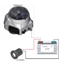
STEP 2 Plug in cig plug an turn on red switch. Beacon will flash and siren will beep 4 times. Siren will now enter standby mode.
