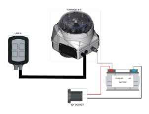
STEP 2 Set up Linx 4, hold down button 1 & 2 and then connect to power. The siren will sound. Refer to MO36 Linx4 installation guide for full instructions. Buttons need to be set to 1= Blue 2= Red 3= Green 4= Amber.
