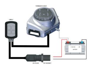
STEP 2 Set up Linx 4, hold down button 1 & 2 and then connect to power. The siren will sound. Refer to MO36 Linx4 installation guide for full instructions. Buttons need to be set to 1= Blue 2= Red 3= Green 4= Amber.
