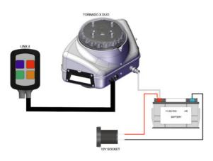
STEP 4 Connect power lead to power and unit will sound 4 beeps (program mode activated)
