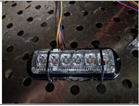
Comments: Device passed IPX9K test with no negative reaction. Lamp worked both at beginning of test cycle, during and after test cycle complete.
