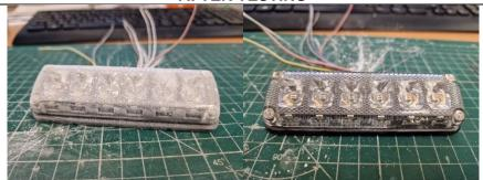
Comments: Device passed IP6X test with no negative reaction. Lamp worked both at beginning of test cycle and after test complete. There was no ingress of dust within the lamp enclosure.
