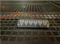
Comments: Device passed test with no negative reaction. Lamp worked both at beginning of test cycle and after test complete.
