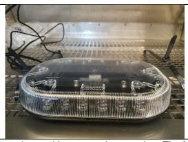
Comments: Device passed test with no negative reaction. The Microbar worked both at beginning of test cycle and after the test was complete.
