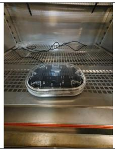
Comments: Device passed IPX9K test with no negative reaction. The microbar worked both at beginning of test cycle, during and after test cycle complete.
