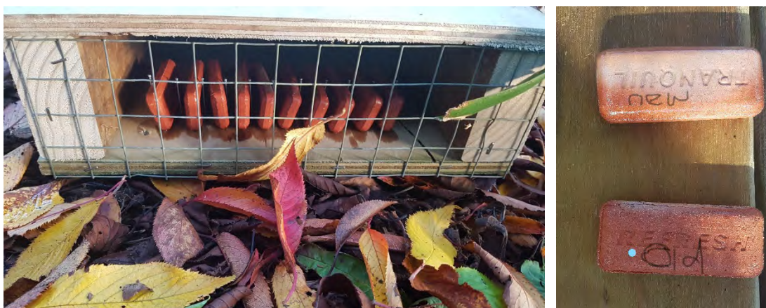
Fig. 3. Left: PoaUku Rat & Possum lure (Lure C) weathering outdoors in a simulated DOC trap box closed off to animal interactions, in preparation for the long-term weathering trials. Right: Comparison between a fresh PoaUku Rat & Possum lure (top) and a 12-week weathered lure (bottom), demonstrating the lack of mould issues.
