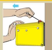
With the palm of one hand pushing against the top surface, use the other to pull the resetting cord firmly toward you until you feel the trap is set.
