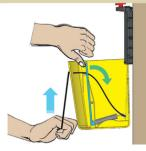
Once you feel it go over centre and start to release, slowly allow the setting cord to be drawn back into the trap, releasing the spring tension, and unsetting
