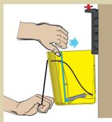
Gently push the back of the protruding bait bar forward, while keeping tension down on the setting cord.
