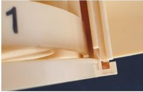
Top part of unit not seated into groove of bottom plate
