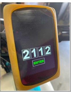
Hold the 'SET' button for 2 seconds to enter the configuration menu. The passcode is 2112. Use 'SET' to save a value and move to the next field, +/- to scroll thru parameter values.
