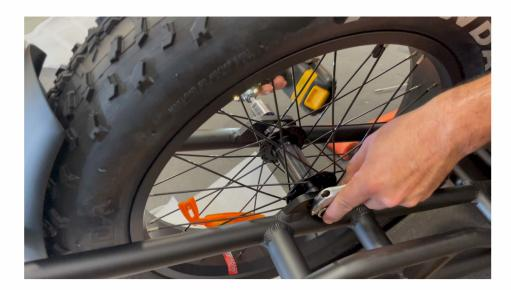
Using 19mm or crescent wrench, hold inner axle nyloc in place while using 19mm socket or driver to tighten outer axle nut. Tighten to 6 foot pounds. Look for even threads on each nut. Wheel should spin freely.
