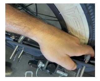
Make sure the shifter cable and main motor cable are free, and are not binding or pinched between the mounting plates, u-bolts, or bike frame.
