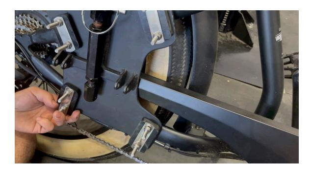
Place rubber caps over the remaining threads on U-bolts
