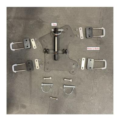
Attach the mounting plate on the right side of bike frame by placing U-bolts around the rear tubes of the frame and through the base plate. The smaller U-bolts go to the rear of the plate, and the wider two go to the front.
