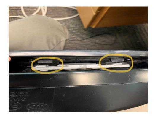
Once bottoms tabs are free, there are two more tabs on the top. You can just wiggle it out by moving the bottom part outward and pulling it down...Carefully.
