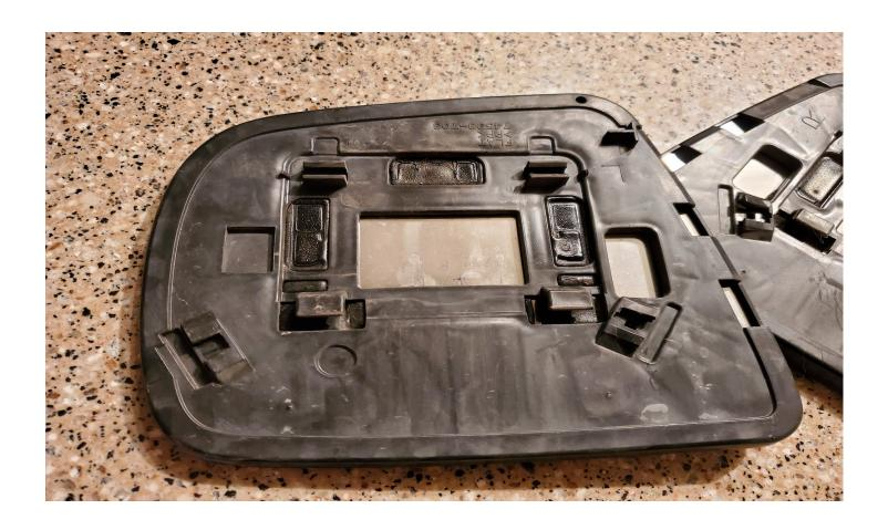
Once the plastic lens case is out, now it's time to take the mirror lens off by heating it up using a heat gun, and a plastic piece to pry the lens off. I normally use a plastic knife (comes with takeout food) but you can also use a plastic trim remover.
