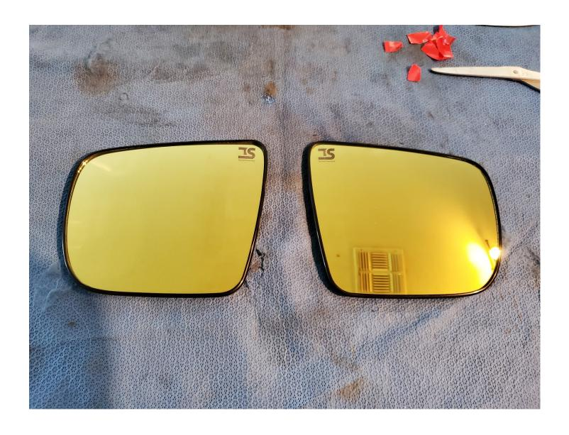
Now you can install the plastic lens piece back with your new Top Shelf lens. Start on putting the top tabs first by sliding it in.
