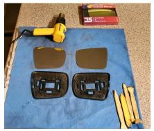
Flip the lens frame back over and gradually pry the frame edges around the edges of the lens. Start in one corner and work your way around. The lens will come right out.
