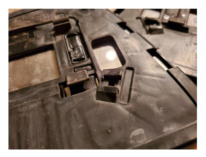
After warming the back of the lens frame, take a plastic trim removal tool and gently slide it between the frame and the lens. This will help separate the lens from the frame.
