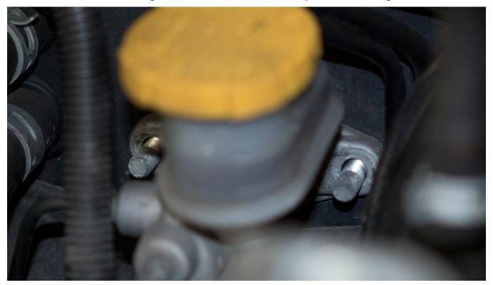
4. With the "U" shaped part of the brace facing towards the driver side of the vehicle, mount the brace underneath the clutch master cylinder using the OEM 2 studs.
