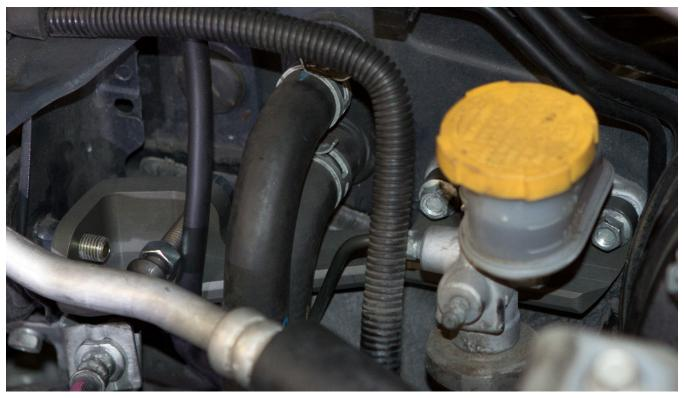
7. Tighten the Pitch stop mount bolt nut and the master cylinder stud nuts evenly.
