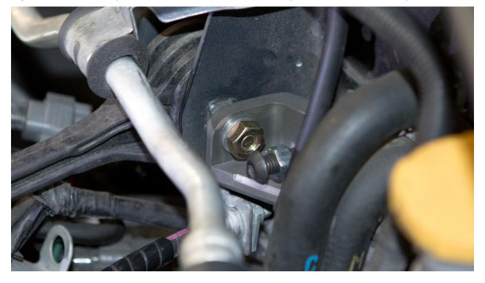
8. Now place the delrin pressure cup on the end of the stainless steel bolt, and tighten the silver nuts so that the delrin cup applies pressure against the firewall. This will keep the brace steady under applied forces from firewall flex.
