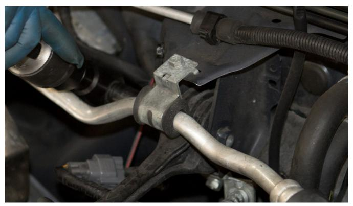
3. Remove the 2 OEM retaining nuts on the clutch master cylinder mounting studs.
