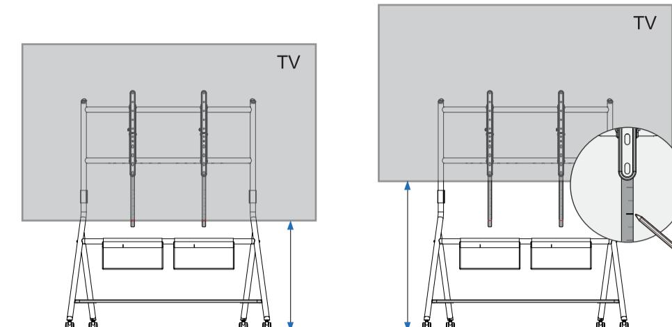
The adjustable range of the distance from the bottom of the TV to the ground is marked on the part 7, so that you can choose the appropriate height. You can choose the height, make a mark on the ruler, and then disassemble and install the part 7 to the back of the TV.
