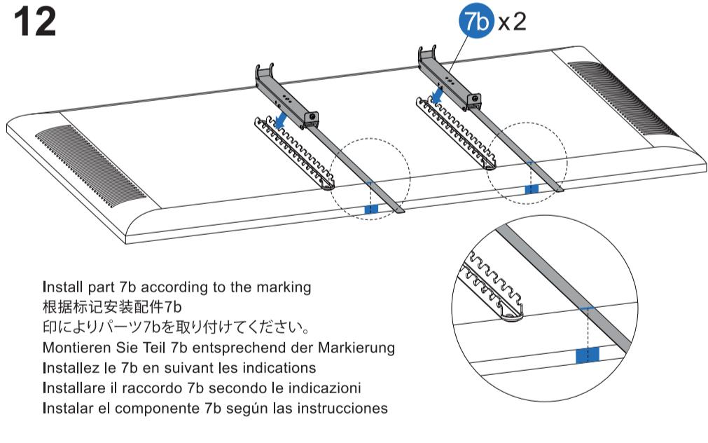
Install part 7b according to the marking
