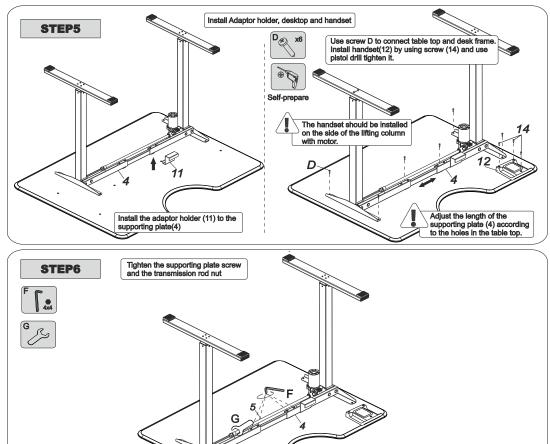
Use a 4x4 allen key(F) to tighten the 4 screws on the supporting plate (4), and then tighten the nut on the transmission rod (5) with a wrench (G).
