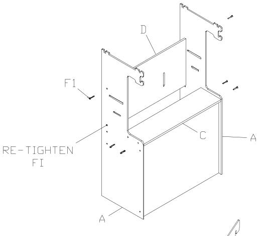
PIVOT COUNTER (D) TO THE UPRIGHT POSITION AND FASTEN USING THE SCREWS REMOVED EARLIER.
