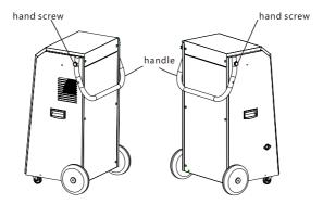
2 2 holes (ABCD) on the left and right sides of the "handle" are aligned with each of the 2 holes (ABCD) on both sides of the machine
