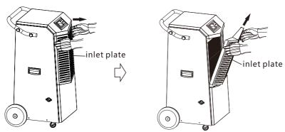
2 As shown in the figure, pull the filter handle with your hand up to about 30mm, then pull down the filter by diagonal.
