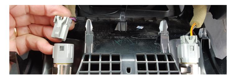
With the fascia free of the vehicle its now time to attach the switch pane to the fascia.
