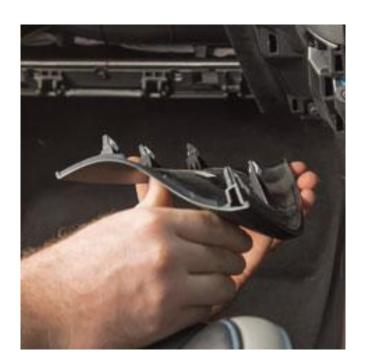
Using the 7mm socket, remove the bolts on either side of the lower centre dash piece.
