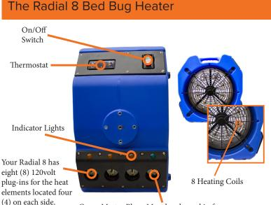
Green Master Plug. Must be plugged in for the machine to operate. Do not plug cords from the PTAC Splitter into this plug!
