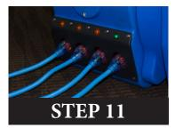
Run additional power cords to the remaining orange plugs. When utilizing wall outlets, make sure the total power draw per circuit does not exceed breaker capacity (2 Blue Cords / 20amp Circuit or 1 Blue Cord / 15 amp Circuit). Note: The green plug is the master plug and should be plugged into a dedicated circuit)
