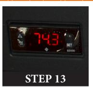
Temperature Controller Your Radial 8 comes with a state of the art digital temperature controller built into the unit. The controller is preset to 132F and requires no need for adjustment to use your Radial 8 unless you want to change the temperature settings. To change the high temperature setting push the set button on the thermostat and use the arrows to adjust temperature up or down. Push the set button when finished.
