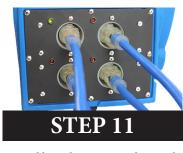
Run additional power cords to the remaining orange plugs. When utilizing wall outlets, make sure the total power draw per circuit does not exceed breaker capacity (2 Blue Cords / 20amp 110 volt Circuit or 1 Blue Cord / 15 amp 110 volt Circuit).
