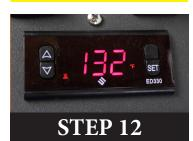
Your Elite 4 Heater comes with a state of the art digital temperature controller built into the unit. The controller is preset to 132° Fahrenheit and requires no need for adjustment to use your Elite 8 unless you want to change the high temperature settings. To change the high temperature setting push the set button on the thermostat and use the arrows to adjust temperature up or down. Push the set button when finished.
