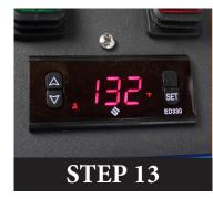
Your Elite 8 Heater comes with a state of the art digital temperature controller built into the unit. The controller is preset to 132° Fahrenheit and requires no need for adjustment to use your Elite 8 unless you want to change the high temperature settings.
