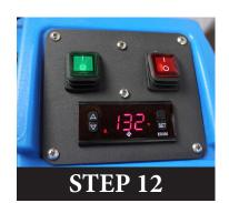
After plugging in all the heating elements, and ensuring all the lights are lit, turn on the fan (GREEN SWITCH), then turn on the heater (RED SWITCH).
