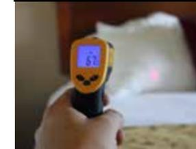
Target temperatures will begin to be achieved around the 7 to 10 hour mark. Monitor the room as desired using the provided infrared laser spectrometer pistol. This will give you a quantifiable measurement of the temperatures in the room. Take temperature readings in the corners, low next to the carpet on the outside walls of the room where glass windows or sliding doors are located. Take temperatures under the bedspread and pillows, inside drawers, around headboards, inside cabinets
