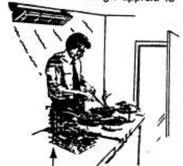
Aim point should be at feet, or on floor behind worker or user.
