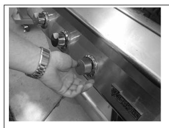
Step 5: Turn on grill burner to high setting to ignite coals. (See Twin Eagles Owner's Manual for proper lighting instructions.)
