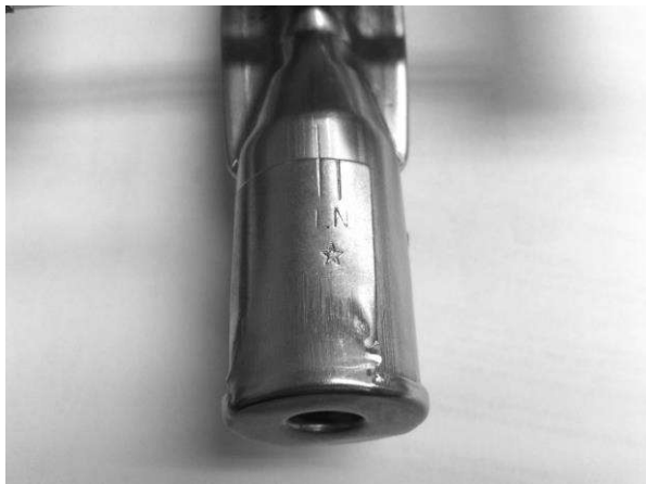
Burner Set at LP
