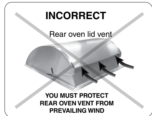
Fig. 8-3 Airflow direction - INCORRECT
