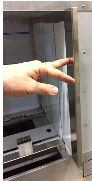
STEP 2: Push Side Filler into place. Repeat procedure for other side.
