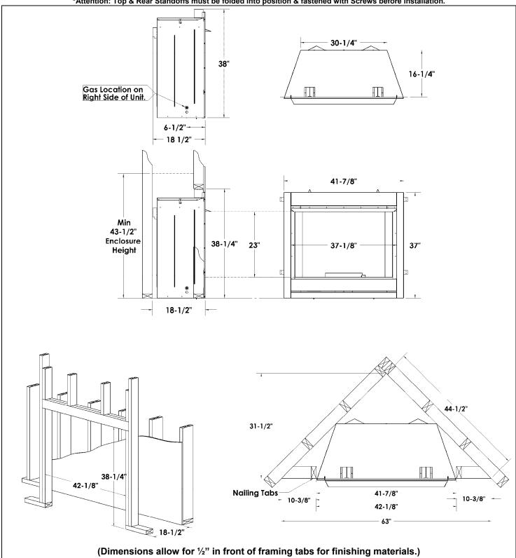
Framing Clearances to Fireplace and Standoffs (Unless otherwise noted): Bottom: 0"/ Sides: 0" / Adjacent side wall: 3-1/2" /Floor of fireplace to ceiling: 7' /Low Profile Enclosure: 43-1/2" Minimum. Back: 0" / Top: 0".
