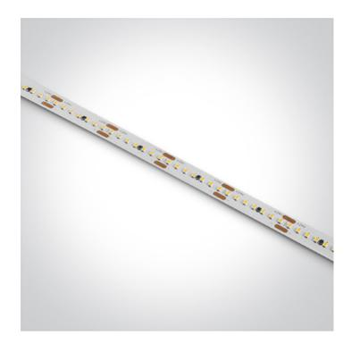
Flexible LED light strip, with SMD2216 LEDs, 238LEDs/meter, 19,2W/meter.Supplied in 5 meters roll with white PCB and double adhesive tape for a better fixing.
