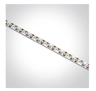
Flexible LED light strip, with SMD2216 LEDs, 300LEDs/meter, 24W/meter.Supplied in 5 meters roll with white PCB and double adhesive tape for a better fixing.
