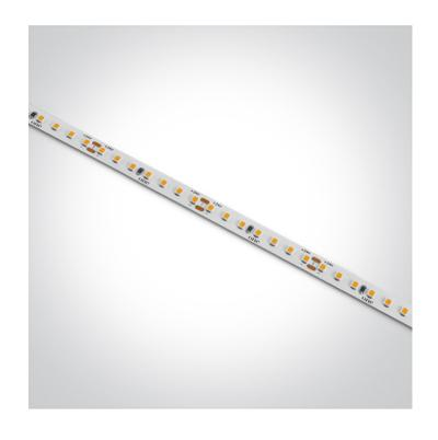
Flexible LED light strip, with SMD2216 LEDs, 140LEDs/meter, 19,2W/meter.Supplied in 5 meters roll with white PCB and double adhesive tape for a better fixing.
