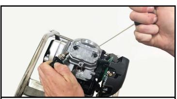
If the plug sparks, reinstall. If the plug does not spark, dry off and pull again, until you see a spark. If the spark plug will not spark, replace the spark plug.
