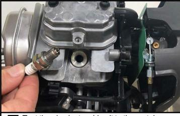
Test the plug by touching it to the metal cylinder & pull the recoil starter several times.
