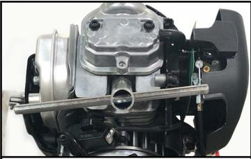
Remove the engine's spark plug with a spark plug wrench.
