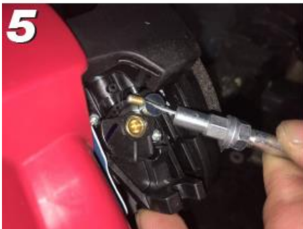
Locate accelerator screw found on HONDA engine and place cable through the gap.
