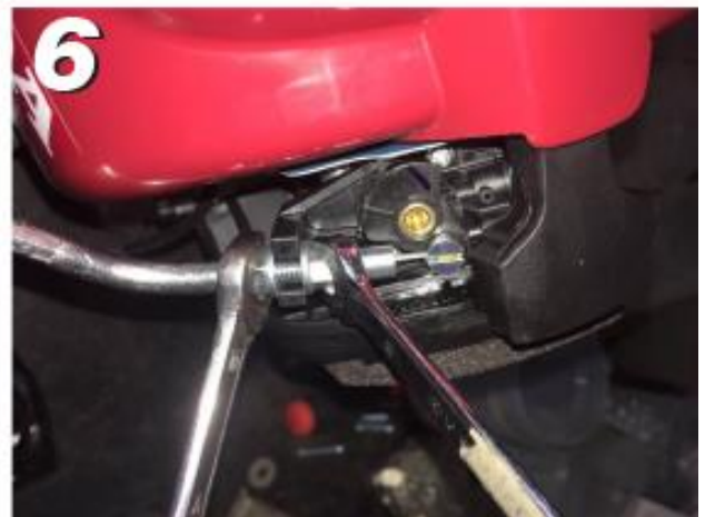
Tighten and make sure that when you pull accelerator handle, the cable engages engine.
