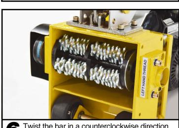
Twist the bar in a counterclockwise direction to tighten (reverse thread).
